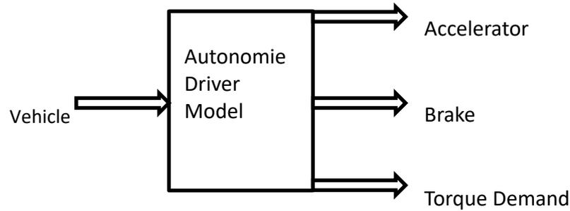
**Figure VI-2 – Autonomie Driver Sub-Model inputs and outputs**
