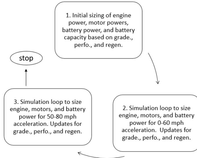
**Figure VI-32 – Simplified SHEVPS Sizing Algorithm in Autonomie**
