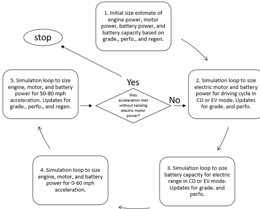
**Figure VI-34 – Simplified PHEV Sizing Algorithm in Autonomie**
