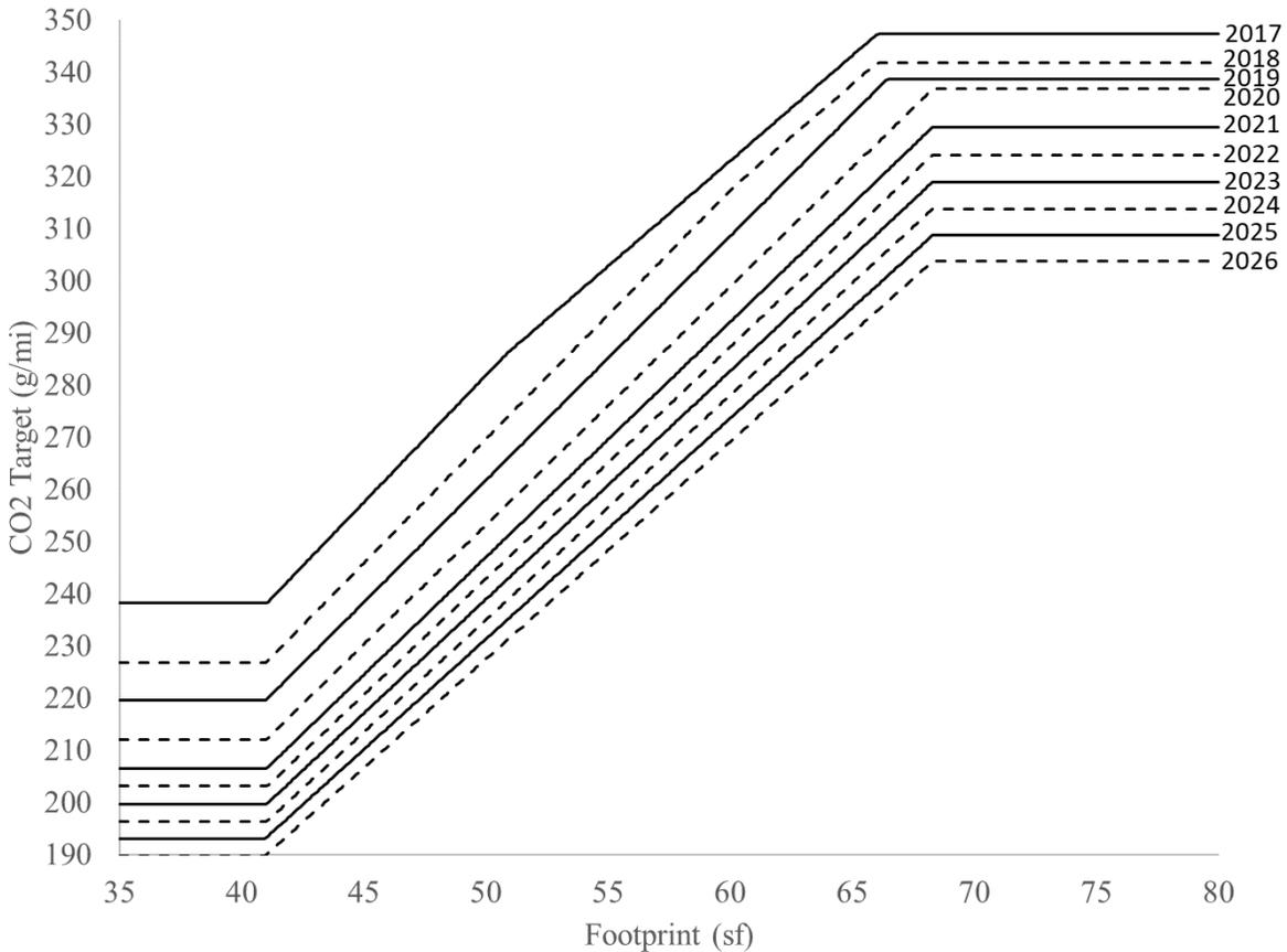
**Figure II-4 – Light Truck CO<sub>2</sub> Targets**
