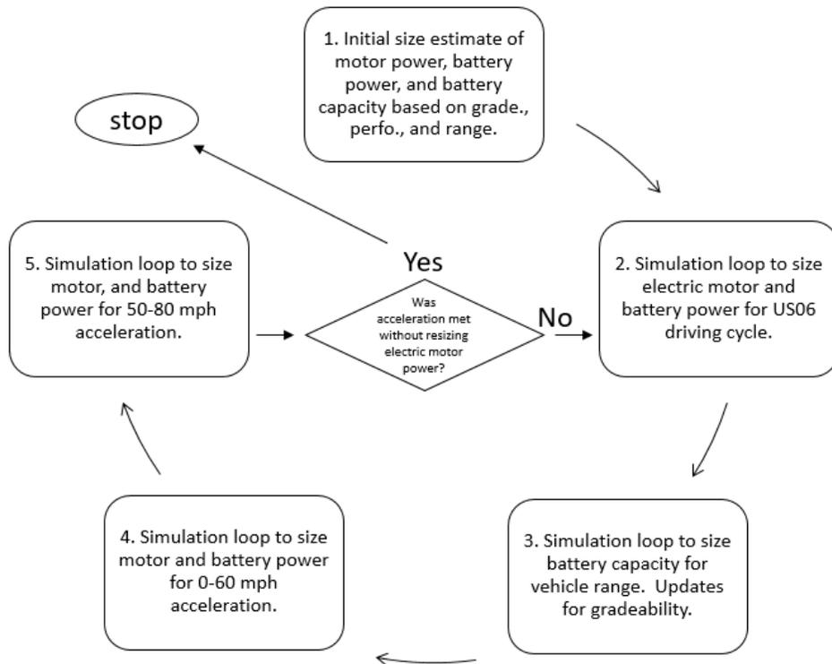
**Figure VI-35 – Simplified BEV Sizing Algorithm in Autonomie**
