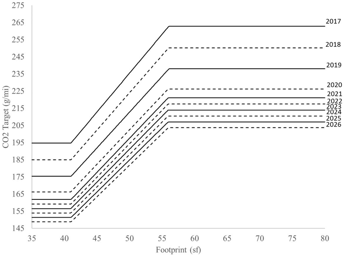
**Figure II-3 – Passenger Car CO<sub>2</sub> Targets**
