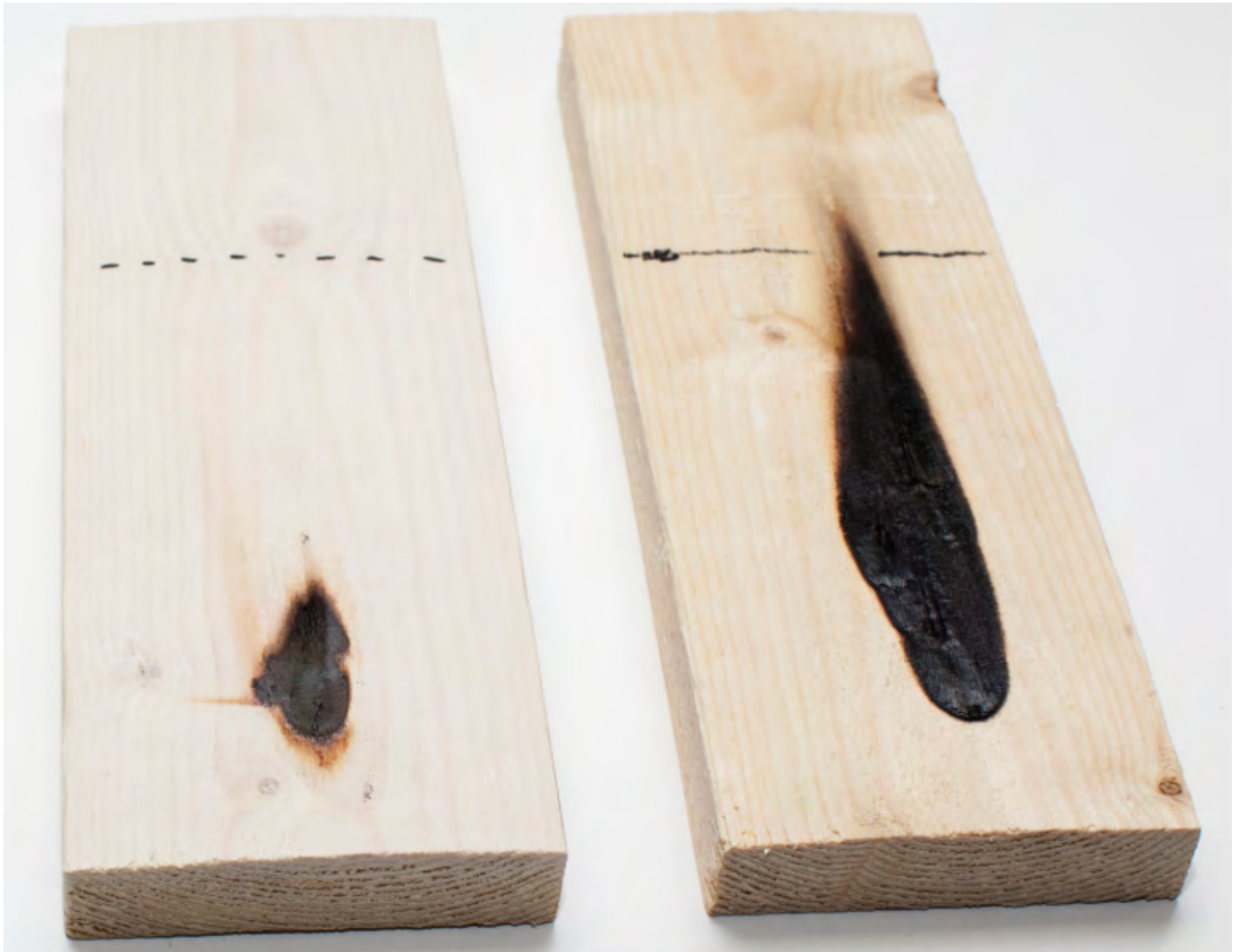
HefCel-coated wood (left) and untreated wood (right) after 30 seconds flame test. (Photo: VTT)
