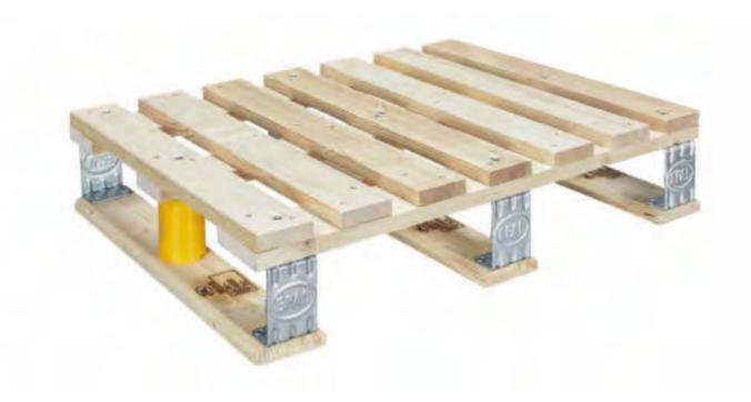
The EPAL 7 half pallet measuring 800 x 600 mm was developed as a quality assured alternative to the "Düsseldorfer" pallet. The addition of round blocks featured in EPAL 7 marks a design update from the previous EPAL half pallet.
