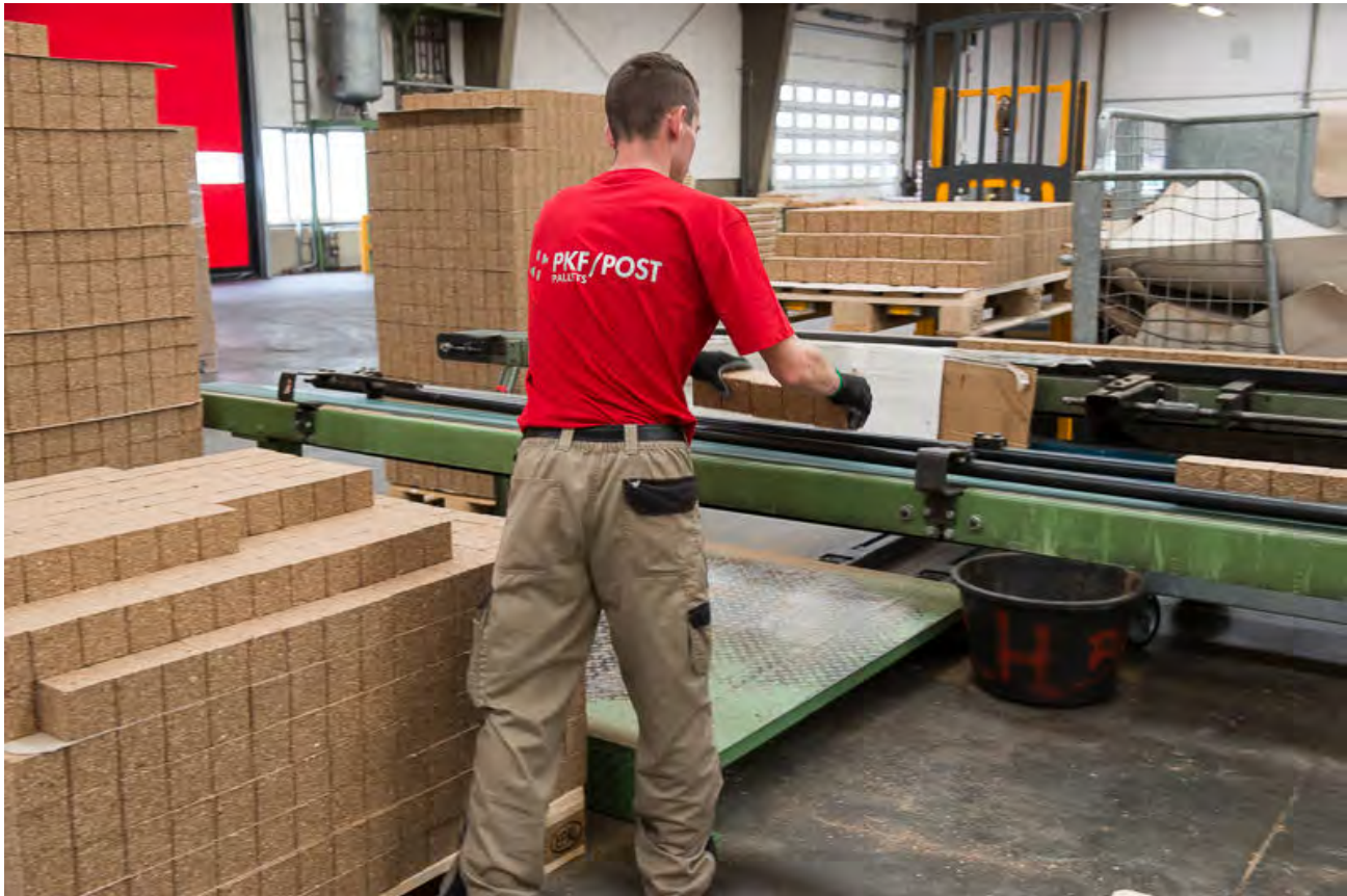
Dimensionally consistent wood composite blocks being fed into an automated nailing system in the Netherlands, as seen on the FEFPEB 2017 plant tour.
