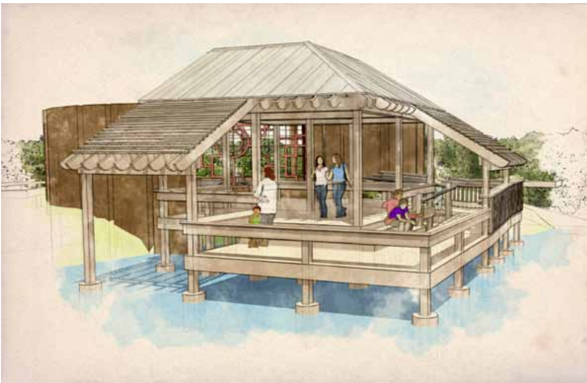
Figure 4: Rendering of Project WET proposed classroom structure overlooking primary wetland unit, on campus of Mississippi State University, 2012. The structure has passive solar features, is fully ADA compliant, and can seat up to 50 students. Graphic by D. Havelin
