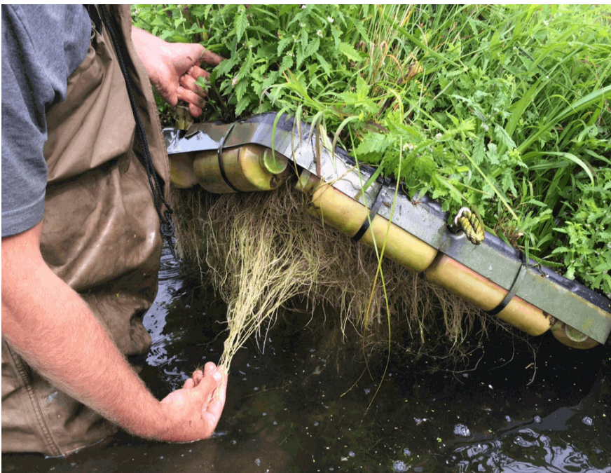
FIGURE 16. PhytoLinks module showing HDPE-encased flotation system.
