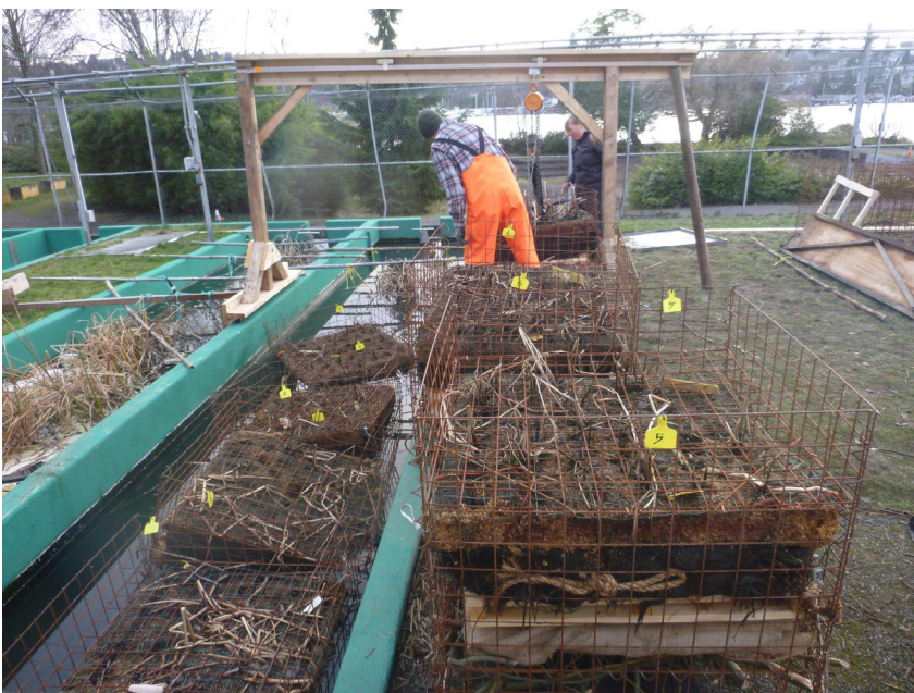
FIGURE 3. Floating wetland biofilter constructed of bio-based substrates protected by untreated gabion basket.
