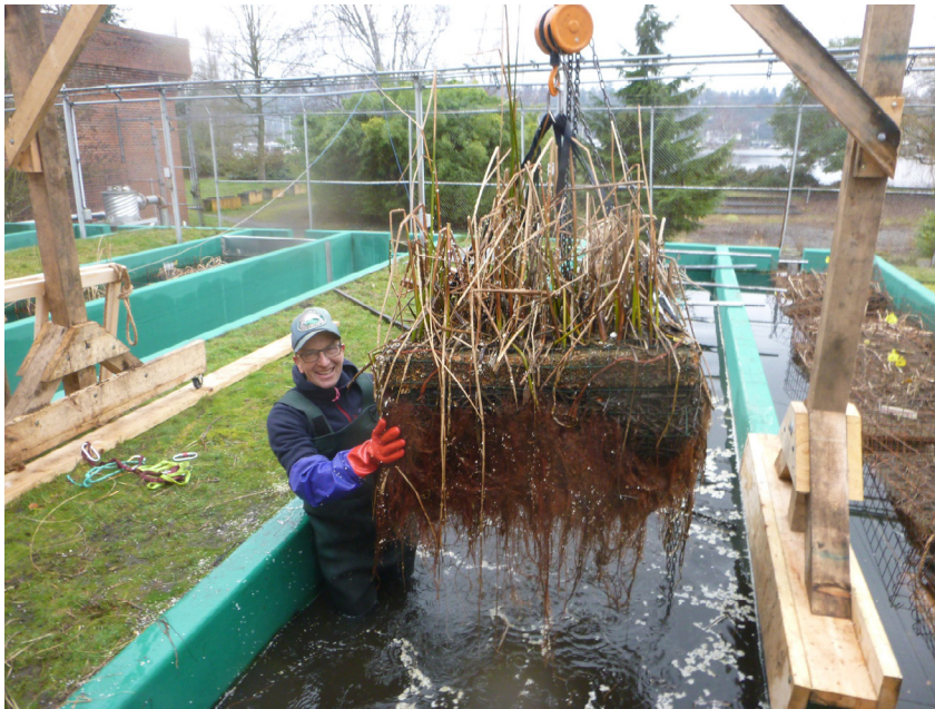
FIGURE 3. Floating wetland biofilter constructed of bio-based substrates protected by untreated gabion basket.
