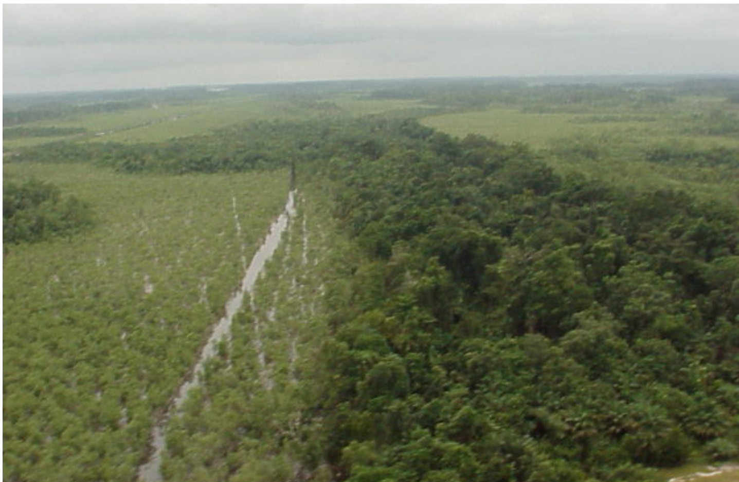
FIGURE 3. Seismic lines across mangrove swamp in the Niger Delta. (Note freshwater swamps beside the mangrove swamp)
