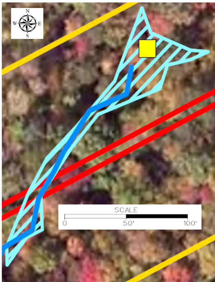
FIGURE 1. Obvious misclassification of forested wetland (pale blue stripes) along a partially identified perennial headwater stream (dark blue) in this excerpt from a July 2015 applicant aerial site plan drawing. Pale blue striped wetland polygon was recorded as palustrine emergent (PEM). Yellow lines show project study area limits; red lines are proposed new pipelines through the mature forest. Yellow box is applicant's wetland data log location for W-L24, where data in Figures 3 and 4 were recorded. The applicant's photobase, other aerial photos, and onsite observations (Figure 2) confirm the applicant's failure to record trees present at the sampling location. This airphoto apparently was taken circa autumn 2013.
