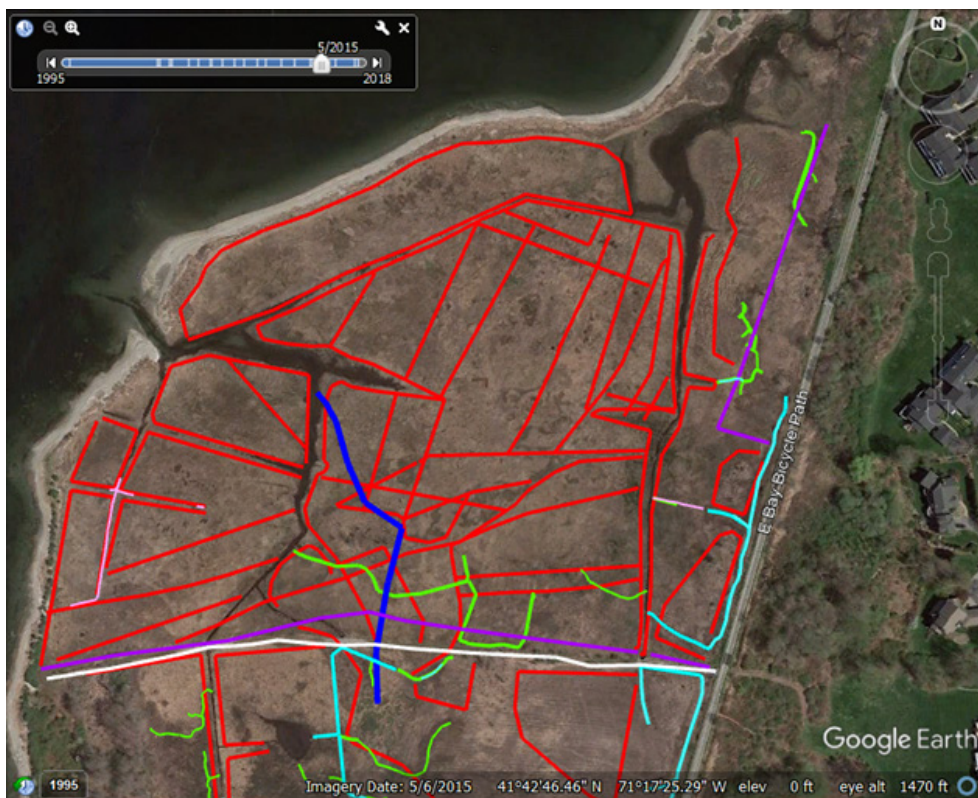
FIGURE 11. Jacob’s Point, Warren, RI, with runnels (light green), larger cleared channels (light blue), ditches (pink), embankments (red), stonewall embankments (purple), road/footpath (white), possible historic channel (dark blue) (Google Earth accessed May 19, 2020). All delineations were based on aerial signatures and need to be field verified.
