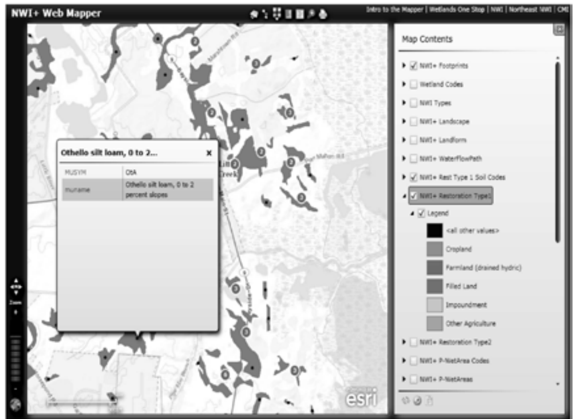
Figure 3: Example of potential type 1 restoration sites with table showing soil type for area of interest. Sites are mostly cropland (drained hydric soil). Numbers in circles represent multiple polygons, zoom in to locate “dots” for accessing soil code.
