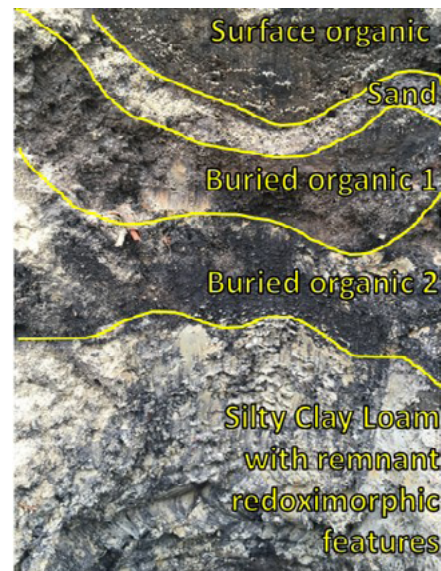
Figure 2. Soils within the Lower Mainland Fraser Valley are often highly disturbed, as shown in this soil profile. Multiple changes to site use, including clearing and drainage for agricultural use, development as a golf course, and commercial development have occurred in this location. This has resulted in new anthropogenic soil horizons (such as the buried sand and buried organic layers) and has altered soil development processes.
