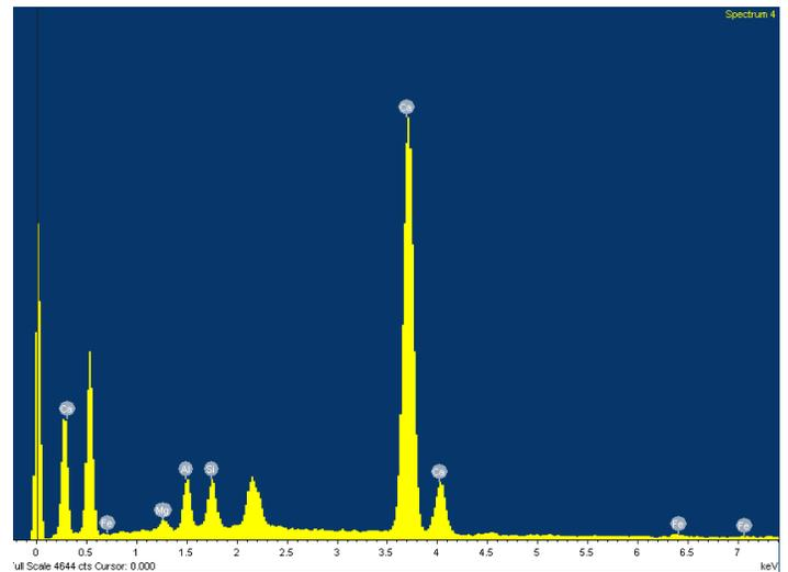
Figure 4. Microscopic view of porosity of a sabana soil. Left: Image taken on a JEOL JSM6360LV Scanning Electron Microscope, 20 kV at 300X. Right: Spectrum with energy dispersive X-ray spectroscopy (EDS) of the sample in the left. This spectrum shows the most abundant elements; calcium, magnesium, silicon, iron, aluminium, chloride. (Photo by Silvia Beatriz Andrade Canto)
