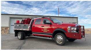
the path of wildfire. This truck is equipped with 400 gallons of water, approximately 20 gallons of foam, wildland fire tools (chainsaws, shovels, picks), and if needed it can be equipped with additional rescue equipment. This new truck has a crew cab and can hold five fire personnel. In 2020 the brush trucks were dispatched 27 times.
