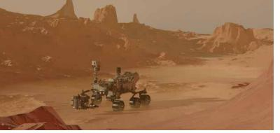
On September 23, 2021, NASA reported that Mars rover, Perseverance had successfully collected and sealed core samples from Jezero Crater. An analytical instrument called SHERLOC and a camera named Watson are attached to the Perseverance, and the data these tools collected and analyzed determined that the Mars samples are of volcanic origin.
