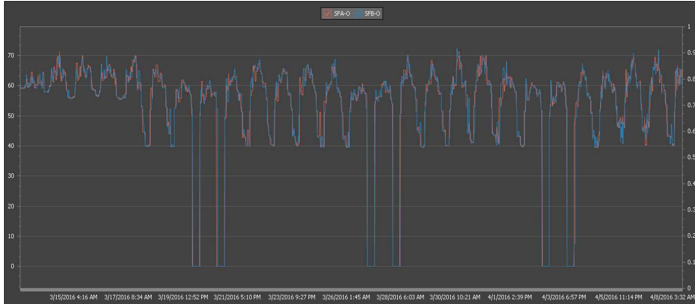
Speed of supply fans post-implementation
