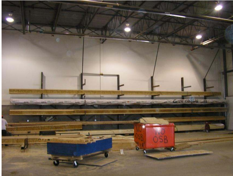
Figure 6: Floor joist inventory in pre-fab plant
