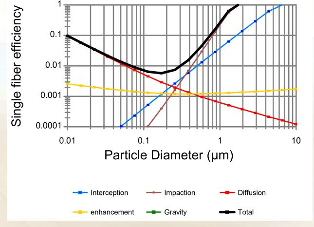
The "most penetrating particle size" is typically in the 0.1-0.3 µm range.
