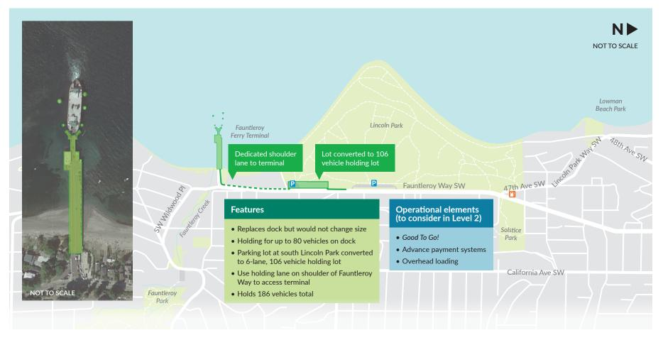
**Alternative A-7** replaces the dock at the same size and location as the existing facility and could hold up to 80 vehicles. This alternative uses the existing south parking lot at Lincoln Park to hold up to 106 vehicles, accommodating a total of 186 vehicles.
