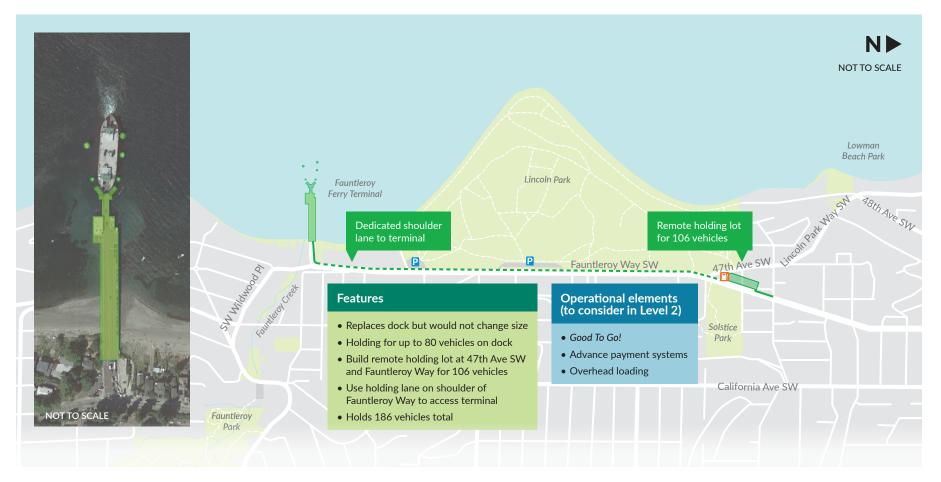
**Alternative A-6** replaces the dock at the same size and location as the existing facility and holds up to 80 vehicles. This alternative includes a remote holding lot near 47th Ave SW that holds up to 106 vehicles to accommodate a total of 186 vehicles.
