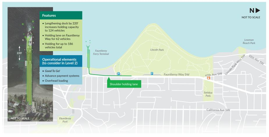
**Alternative B** replaces the dock with a longer dock that could hold up to 124 vehicles. Fewer cars would need to line up outside the terminal, so the holding lane on Fauntleroy Way shows a line of 62 vehicles to accommodate a total of 186 vehicles.
