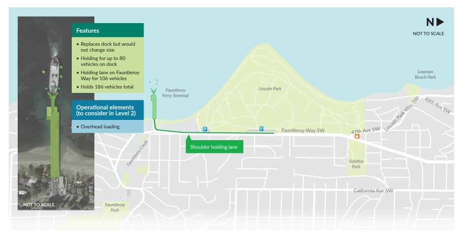
**Alternative A-1** replaces the dock at the same size and location as the existing facility and could hold up to 80 vehicles, with the shoulder holding lane the same length as it is today to accommodate a total of 186 vehicles.
