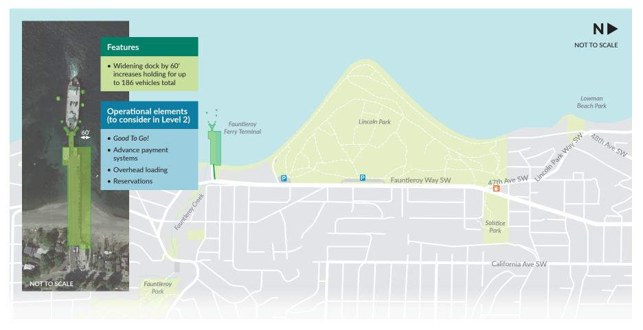
**Alternative C** replaces the dock with a wider dock that could hold up to 186 vehicles without vehicles lining up on Fauntleroy Way. This alternative improves operational efficiency by holding more vehicles on the dock.
