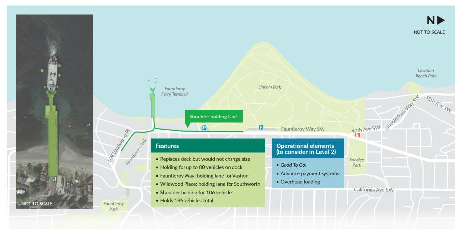
**Alternative A-5** replaces the dock at the same size and location as the existing facility and could hold up to 80 vehicles. To support vehicle processing, this alternative includes separate approach routes and vehicle holding for the two destinations served by the Fauntleroy terminal. Vehicles traveling to Vashon Island would line up along Fauntleroy Way and vehicles headed to Southworth would access the terminal from SW Wildwood Place.
