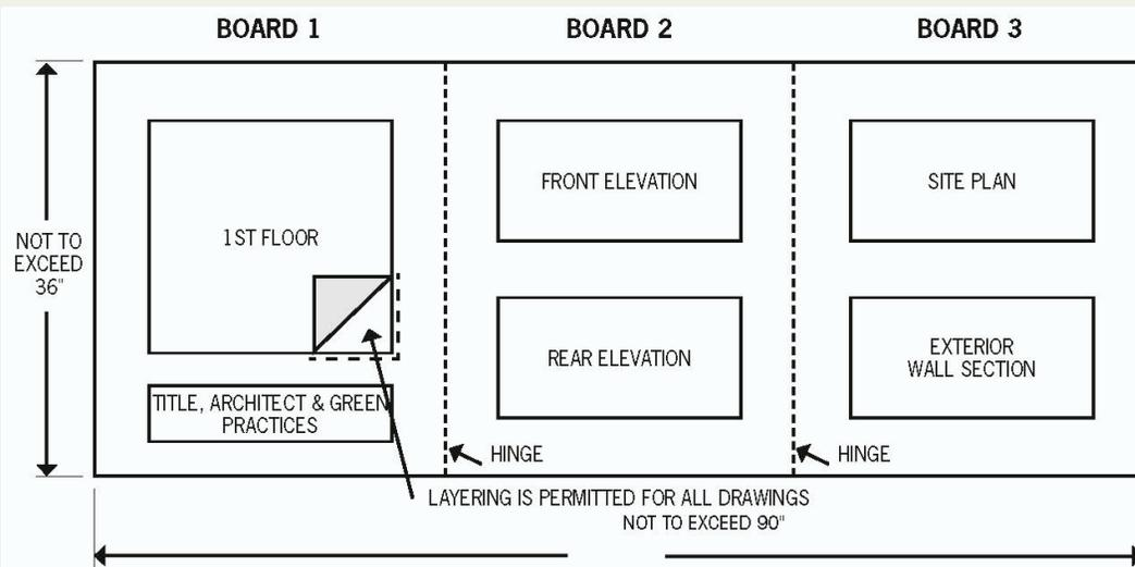
**This sample entry board layout must be used. When opened, boards should measure no more than 36 inches tall by 90 inches wide.**
