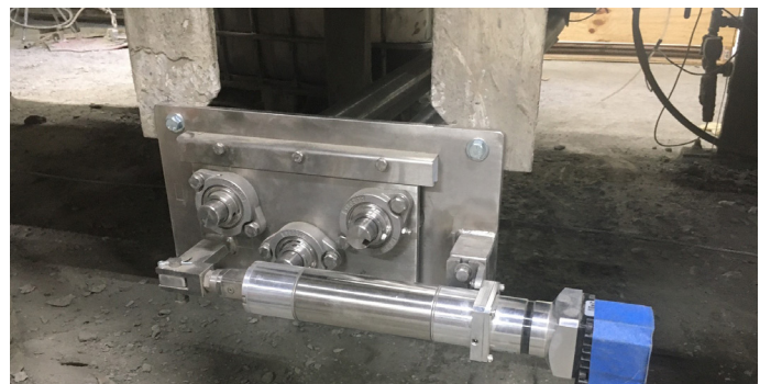
Servomotor actuator for a three roll tracker.
