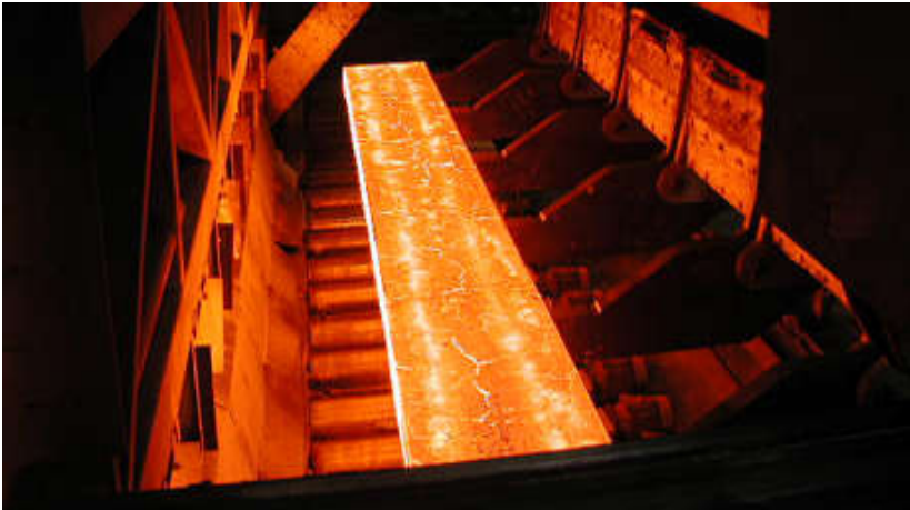
Reheat Furnace: heat slab to proper rolling temperature 2100 – 2350°F
