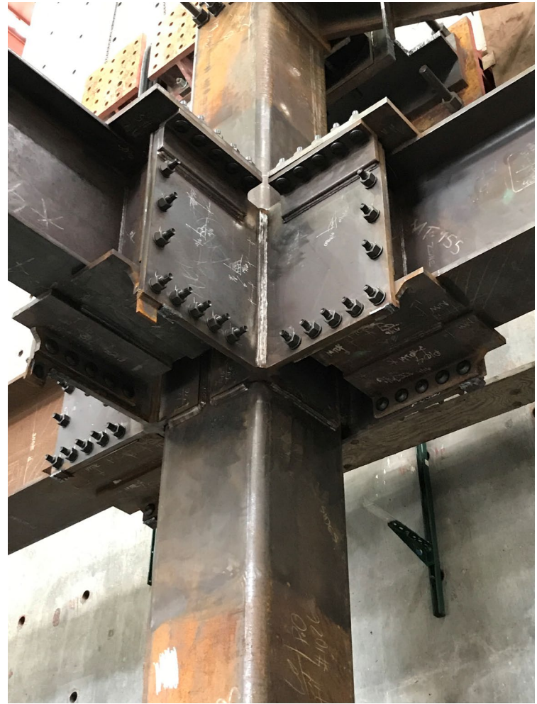
SIDEPLATE SYSTEMS AND COREBRACE TESTING
