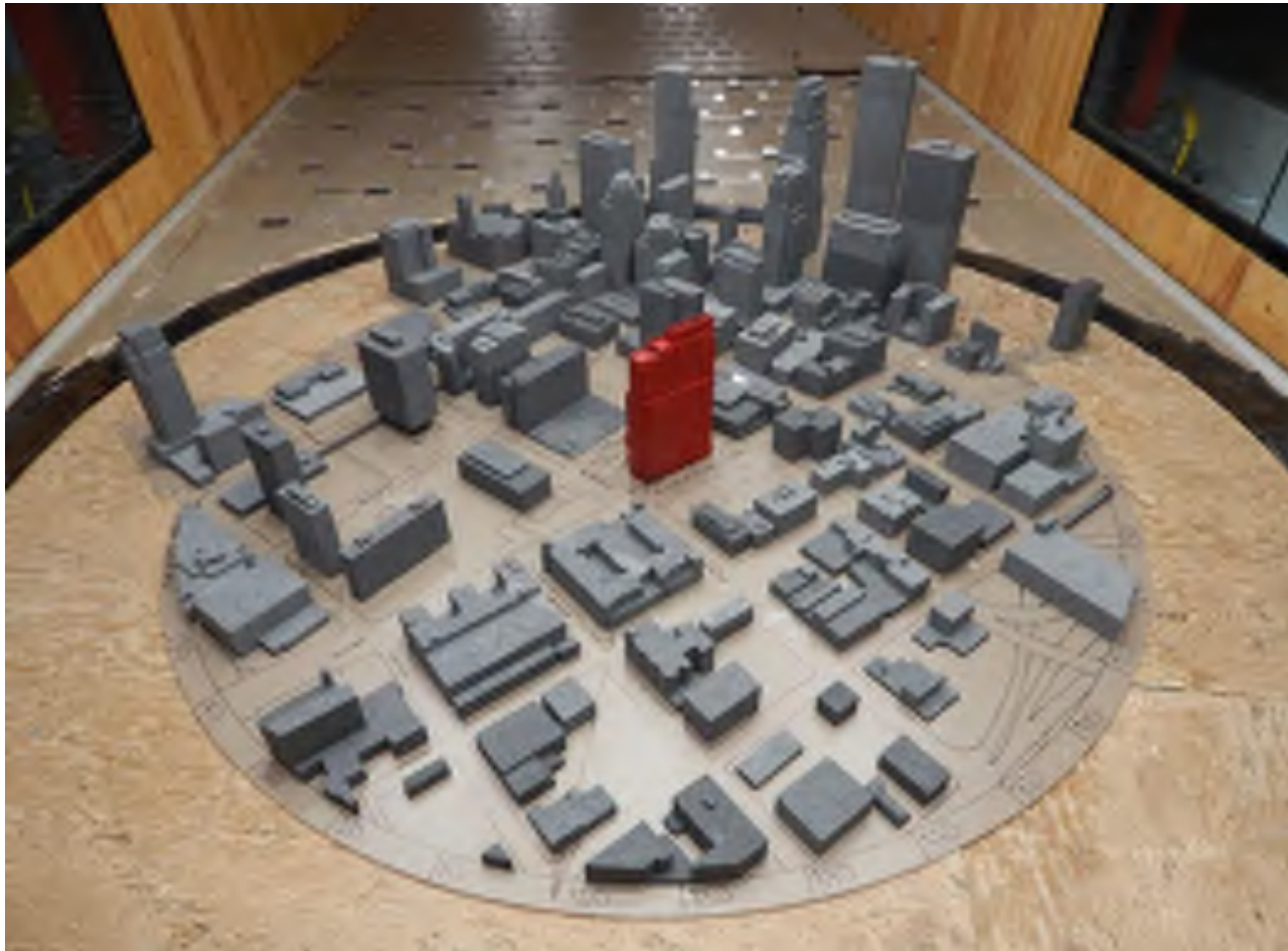
WIND TUNNEL STUDY MODEL – 1:400 SCALE MODEL OF RBC GATEWAY BUILDING WITH MODELS OF SURROUNDING BUILDINGS WITHIN 1,500 FEET
