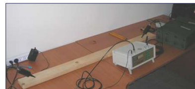
ASTM C597: Test Method for Pulse Velocity Through Concrete
