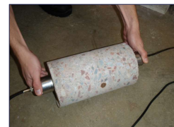
ASTM C597: Test Method for Pulse Velocity Through Concrete
