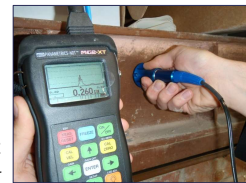
Steel: ultrasonic thickness meter
