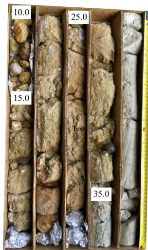
Figure 2. Core sample of glacial sediments collected from a location in Illinois. The core box is 2 feet long, holding a maximum of 10 feet of core length. The top depth of the recovered interval is 10 ft while the bottom depth of the recovered interval is 37.5 ft, indicating 27.5 ft of unrecovered core material.
