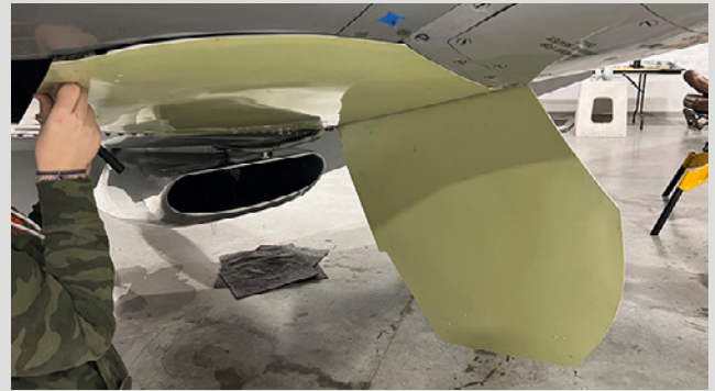
Above: New doors fitted on Val Halla
