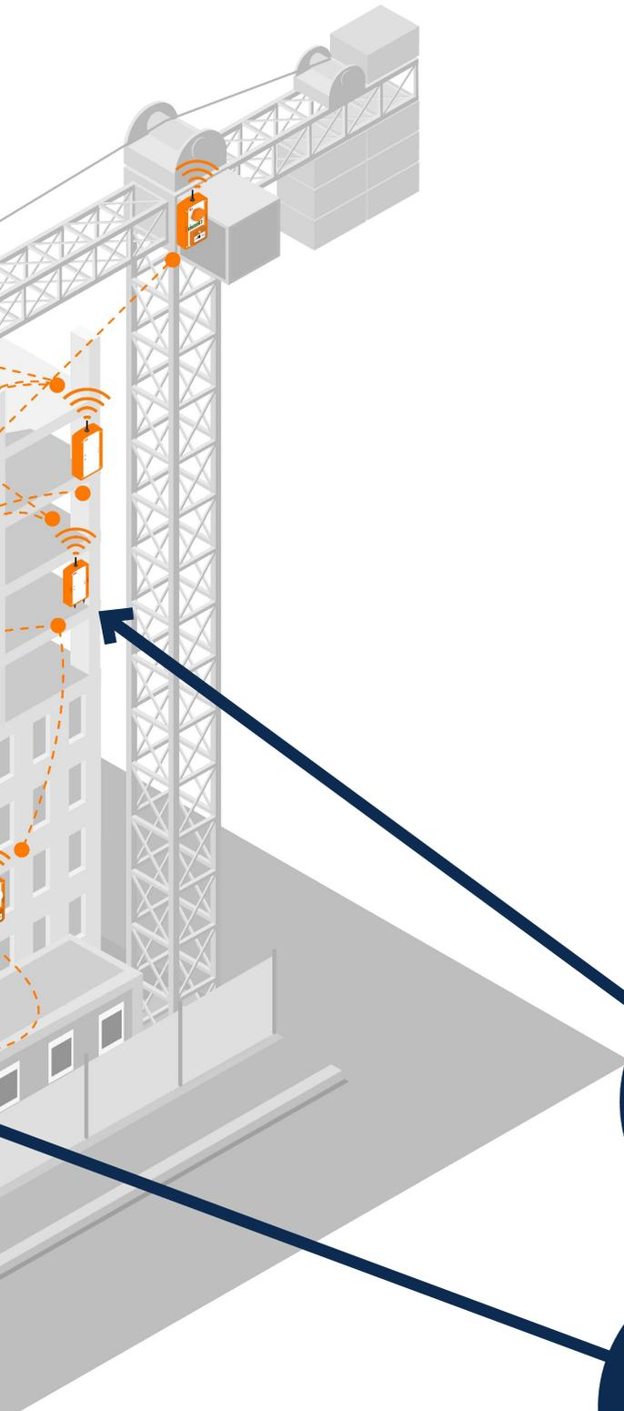
Units are placed in accordance with your fire plan – usually at each stairwell or elevator shaft – and can be added as the build progresses. Units can be numbered according to your fire plan for easy identification in the event of any issues. Heat, smoke or unique dust resistant smoke detectors provide active fire protection in enclosed areas.
